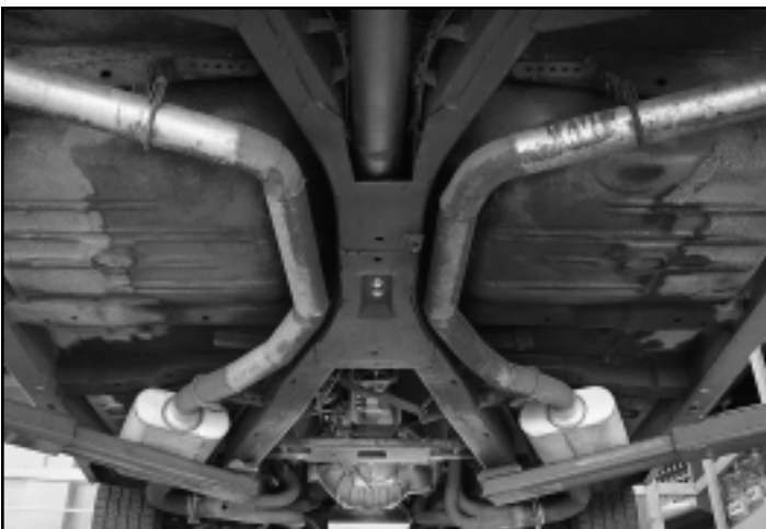
The B-bodies from 1958 to 1964 had an X-frame. The frame came together in the center of the car. This frame flexes easily and would need to be extensively modified for handling purposes.
